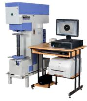
500 to 3000 kgf in steps of 250kgf. • Machine Test height x Throat is 380 x 200 mm. • Fully computerized system for indentation measurement and display. • Windows based software system. • Accurate measurement of Brinell hardness through matched Optics, CCD Camera, Hardware & Software using advanced image processing technology. • Two modes of measurement - Manual & Auto. • In Auto mode the image is scanned for measurement & hardness is displayed automatically.
